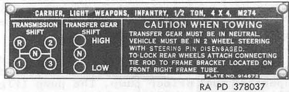
Figure 14. Instruction plate located on top of platform at right of driver - M274 vehicle.
