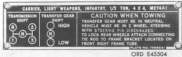
Figure 15. Instruction plate located on top of platform at right of driver - M274A1 vehicle.
